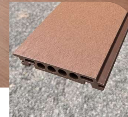
Bamboo Composite Decking - Elegant 2900mm (L) x 140mm (W) x 23mm (T) Weight: 2.83 kg/m
